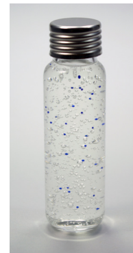
Transparent gel formulation with stabilised beads and gas bubbles
