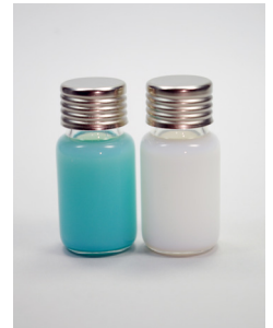
Suspension of Nanoparticles ZnO:Cu (green) ZnO (white)
