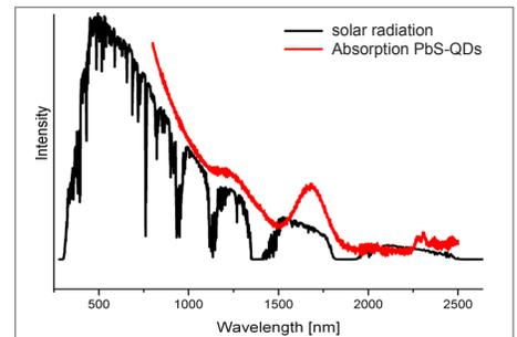
Comparison of solar radiation and absorption spectrum of CANdot® Series C (sketch)
