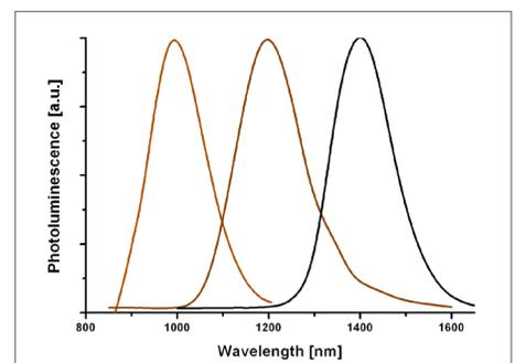
Emission spectra of CANdot® Series C QDs with a maximum at 1000, 1200 and 1400 nm
